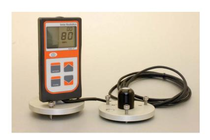
Pyranometers use a silicon cell photodiode and are calibrated to measure total shortwave radiation. The cosine-corrected sensor is designed to maintain its accuracy when radiation comes from low zenith angles.
