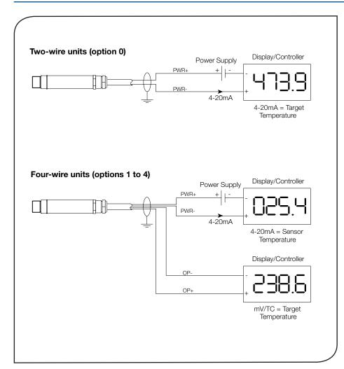
The PyroCouple Series is a range of high quality, low cost, compact sensors which measure the temperature of inaccessible or moving objects and materials. They measure temperatures from -20°C to 500°C, accurately and consistently, with an outstanding response time of 240 ms.
