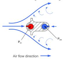
The measurement is done over several measuring points inside the probe. The number of measurement points depends on the duct size and shape. The IML can determine the average air flow volume on the basis of the measurements. The measuring profile shape makes it possible to make accurate measurements from 1.0 m/s air speeds.
